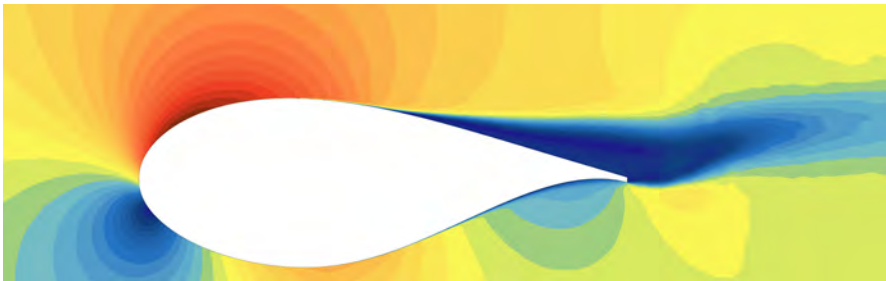
Figure 3: Velocity field of a thick airfoil at high angle of attack with and without an installed vortex generator.
