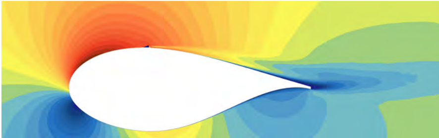
Figure 3: Velocity field of a thick airfoil at high angle of attack with and without an installed vortex generator.
